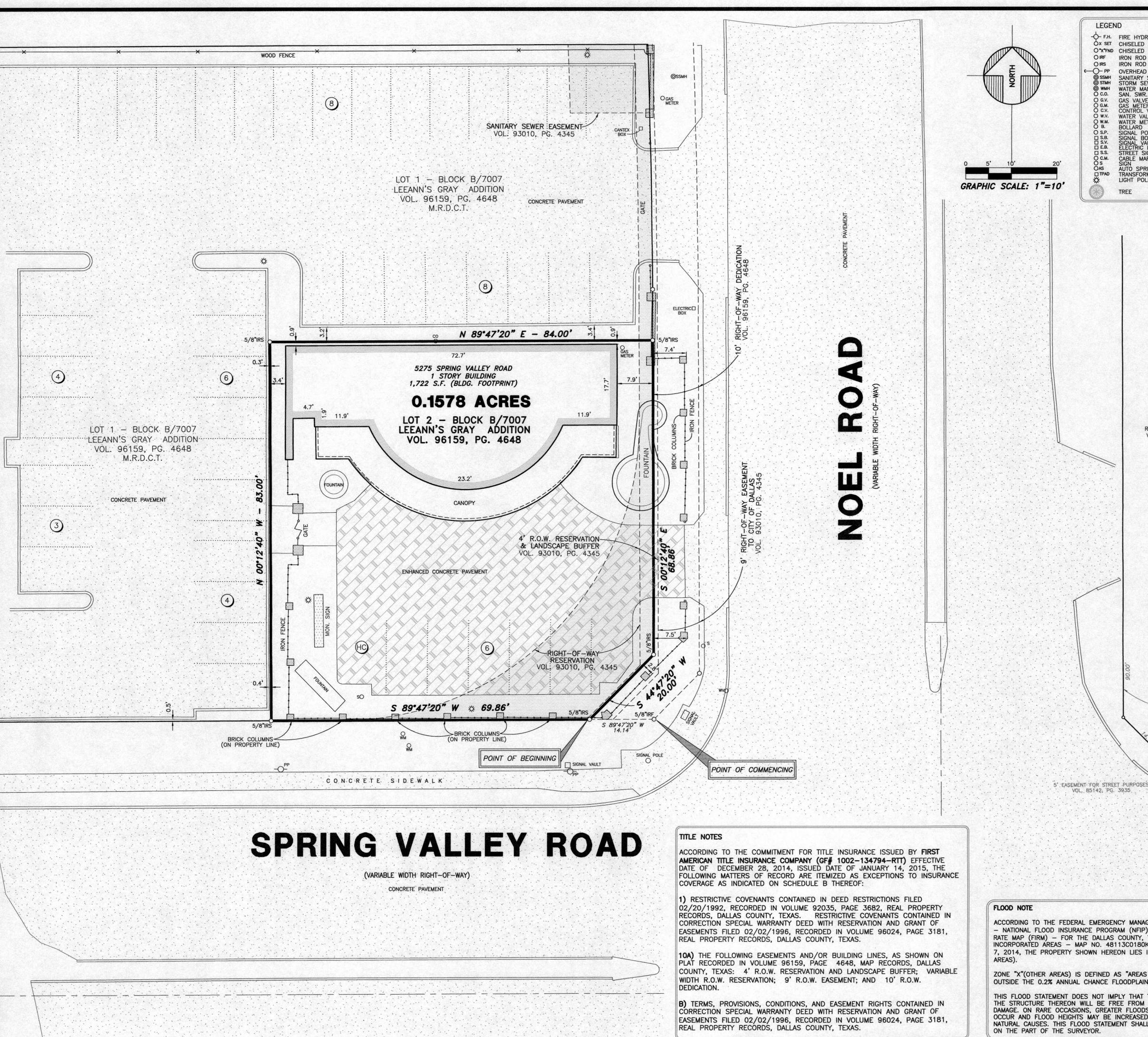
LEGEND -O- F.H. FIRE HYDRANT OX SET CHISELED "X" SET O"x"FND CHISELED "X" FOUND O IRF IRON ROD FOUND (SIZE AS NOTED) OIRS IRON ROD SET (SIZE AS NOTED) O-PP OVERHEAD UTILITY POLE W/ GUY SANITARY SEWER MANHOLE STORM SEWER MANHOLE WATER MANHOLE SAN. SWR. CLEAN OUT O G.V. O G.M. O C.V. O W.V. GAS VALVE GAS METER CONTROL VALVE WATER VALVE SIGNAL POLE SIGNAL BOX SIGNAL VAULT LECTRIC BOX CABLE MARKER SIGN AUTO SPRINKLER TRANSFORMER PAD
