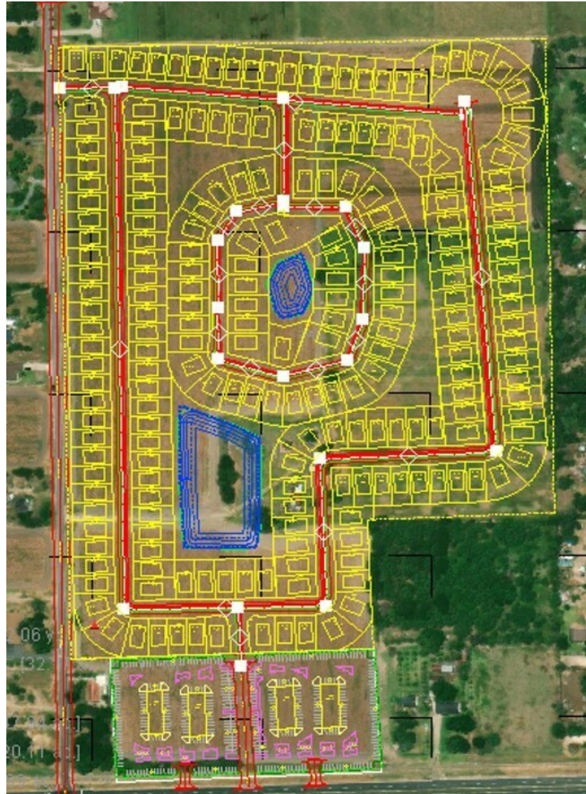
Conceptual layout WITHOUT survey 216 SF LOTS, 110'X50 ON AVERAGE, WITH COMMERCIAL PAD SITES ON HWY 83
