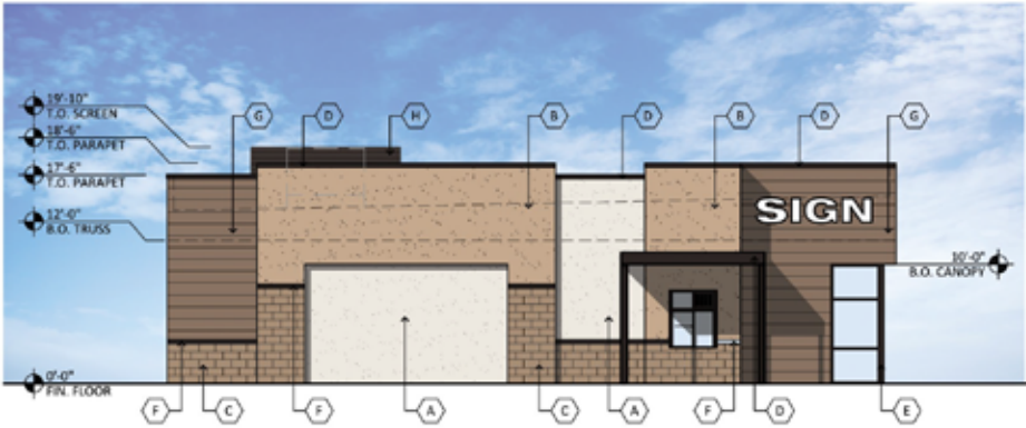
2 NORTH ELEVATIONS SCALE: 3/16" = 1'-0"
