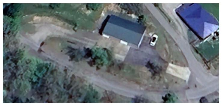
This is an aerial shot showing the concrete driveway at the bottom, the asphalt parking area, the concrete apron at the building, and the drive through and turn around for trucks.
