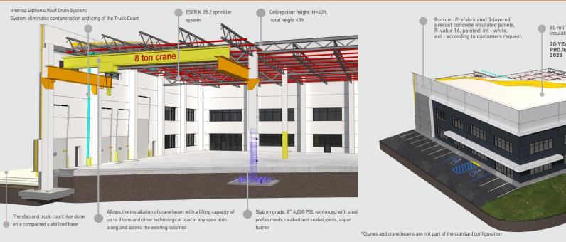
60 mil TPO Extreme R-25 insulation **30-YEAR WARRANTY ON ALL** PROJECTS STARTING FROM 40,000lbs lifting capacity installed in prefab precast
