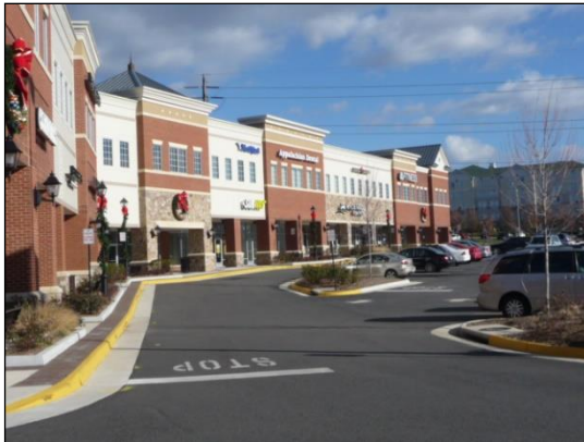
Figure 1228-F: Parapet walls with cornice treatments are used to disguise flat roofs. The image on the right illustrates a tall, thin parapet wall that is prohibited.
