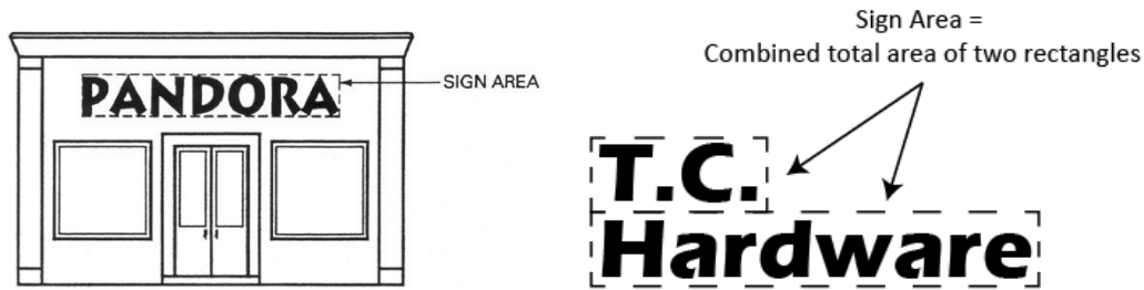
Figure 1236-D: Illustration of sign area calculation for two differently shaped wall signs with individual letters.
