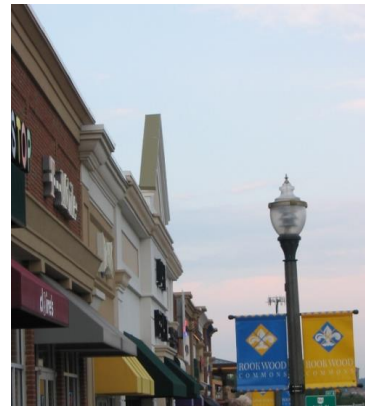
Figure 1228-F: Parapet walls with cornice treatments are used to disguise flat roofs. The image on the right illustrates a tall, thin parapet wall that is prohibited.
