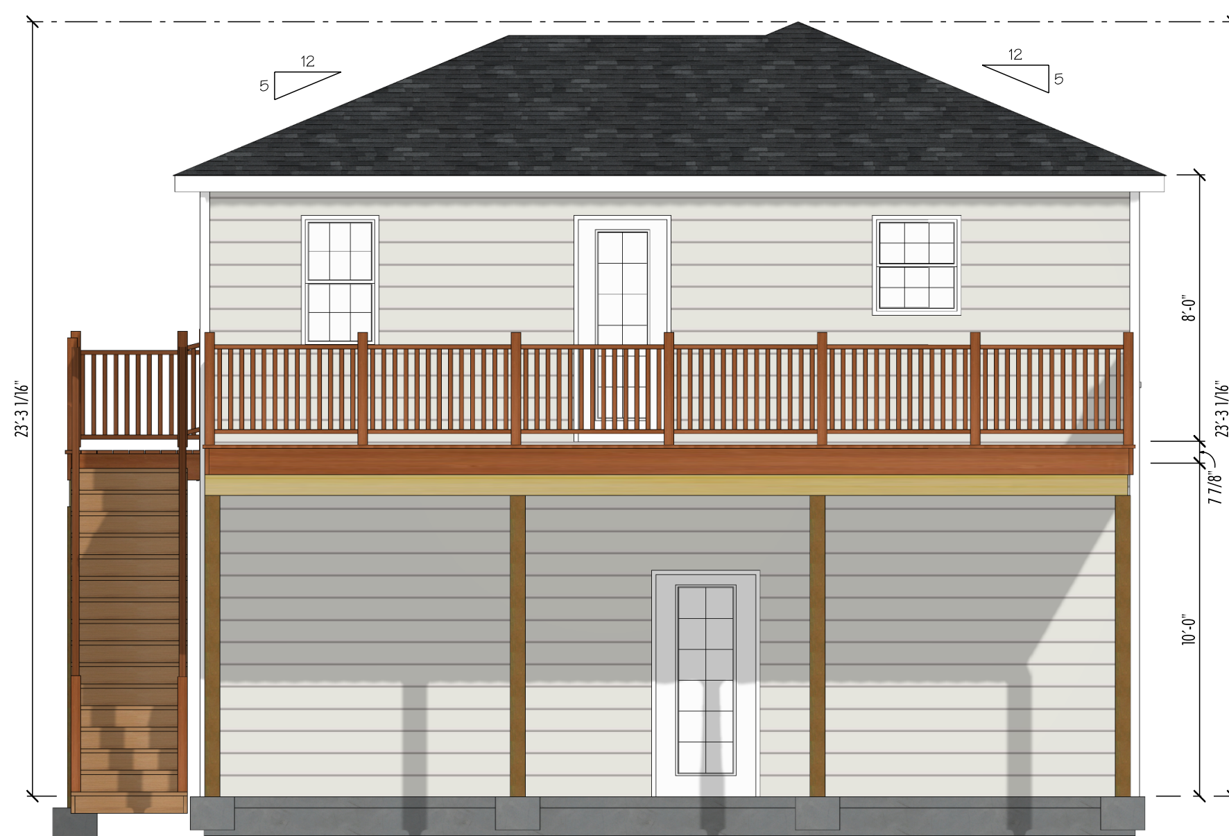
Rear Elevation SCALE: 1/4" = 1'-0"
