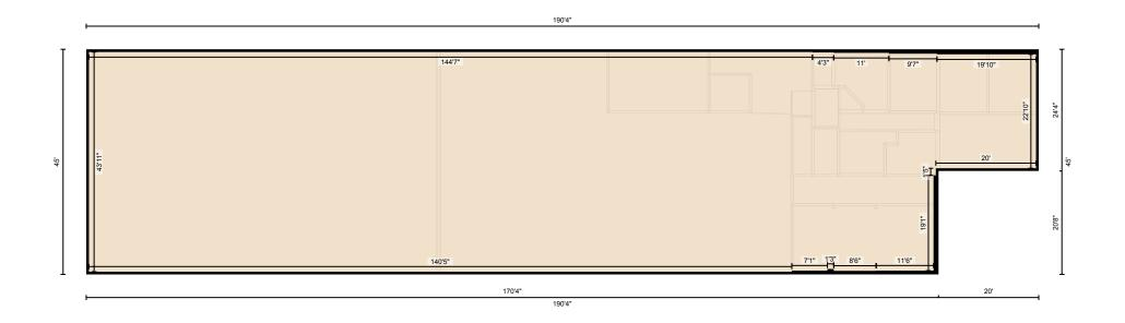
Measurement Diagram for: 2nd Floor Exterior Wall Thickness: 6.5 in
