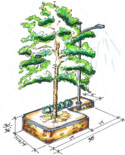
Example of how an island can accommodate both a tree and a light pole
