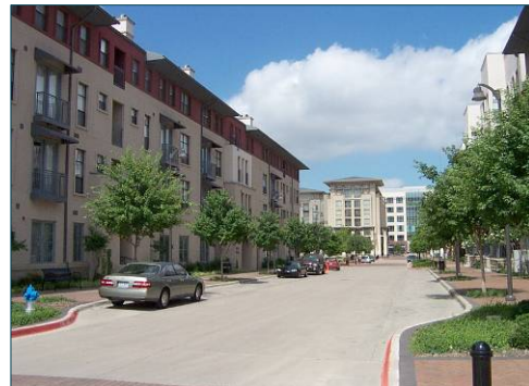
Variation in street width with the use of neck-downs and bulb-outs slows the pace of traffic.
