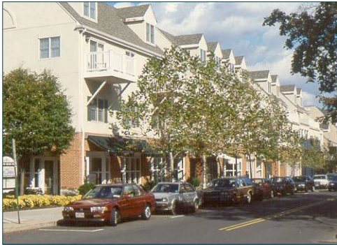
Straight-in, diagonal, or parallel parking should be provided along corridors of high pedestrian activity.
