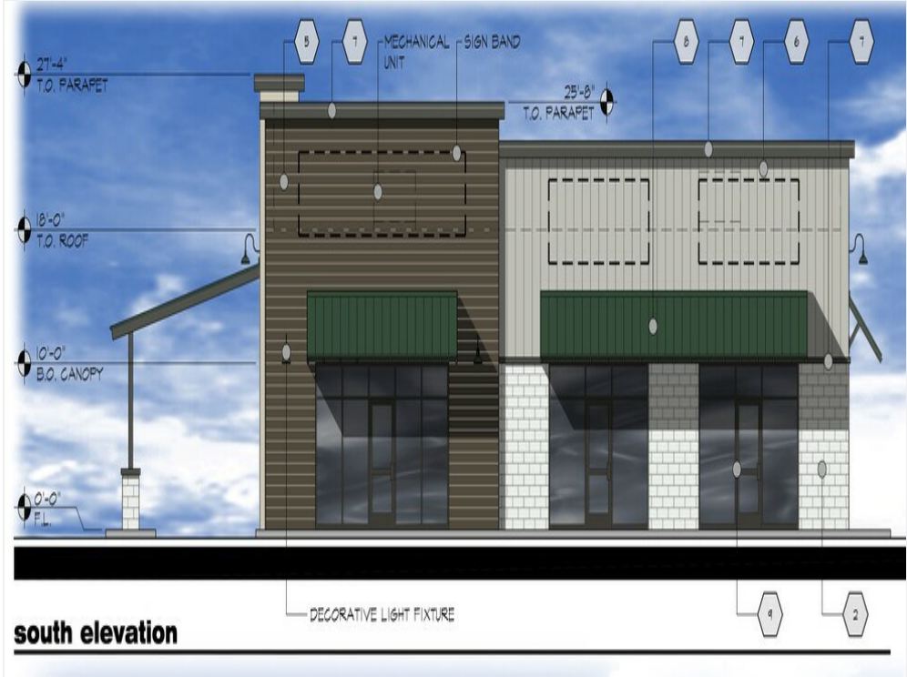
PAD C South Elevation
