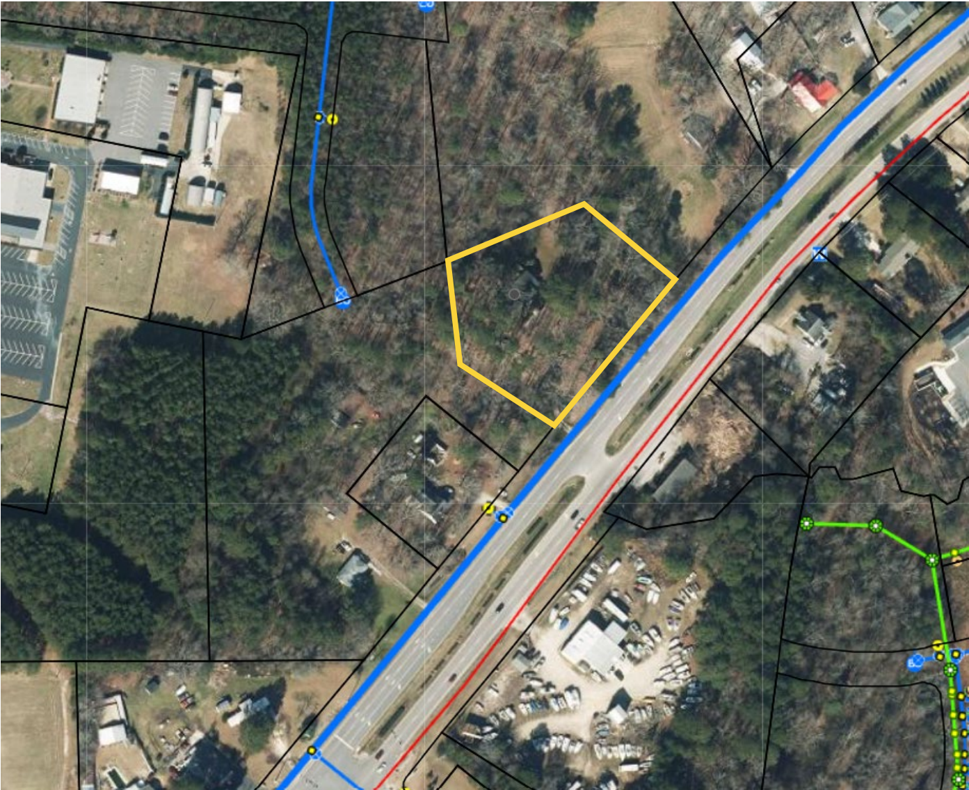
16" water main in the ROW of Knightdale Blvd
