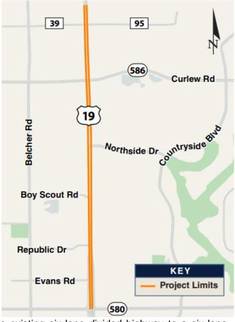
39 project. The \$242.6 million project is modifying the existing six-lane divided highway to a six-lane controlled access roadway with one-way frontage roads in both directions that parallel US 19 from SR 580 to the north of CR 95/CR 39. In addition, new interchanges will be constructed just north of Boy Scout Road and at SR 586 (Curlew Road) to improve traffic flow and safety along this corridor. Estimated project completion is 2029.
