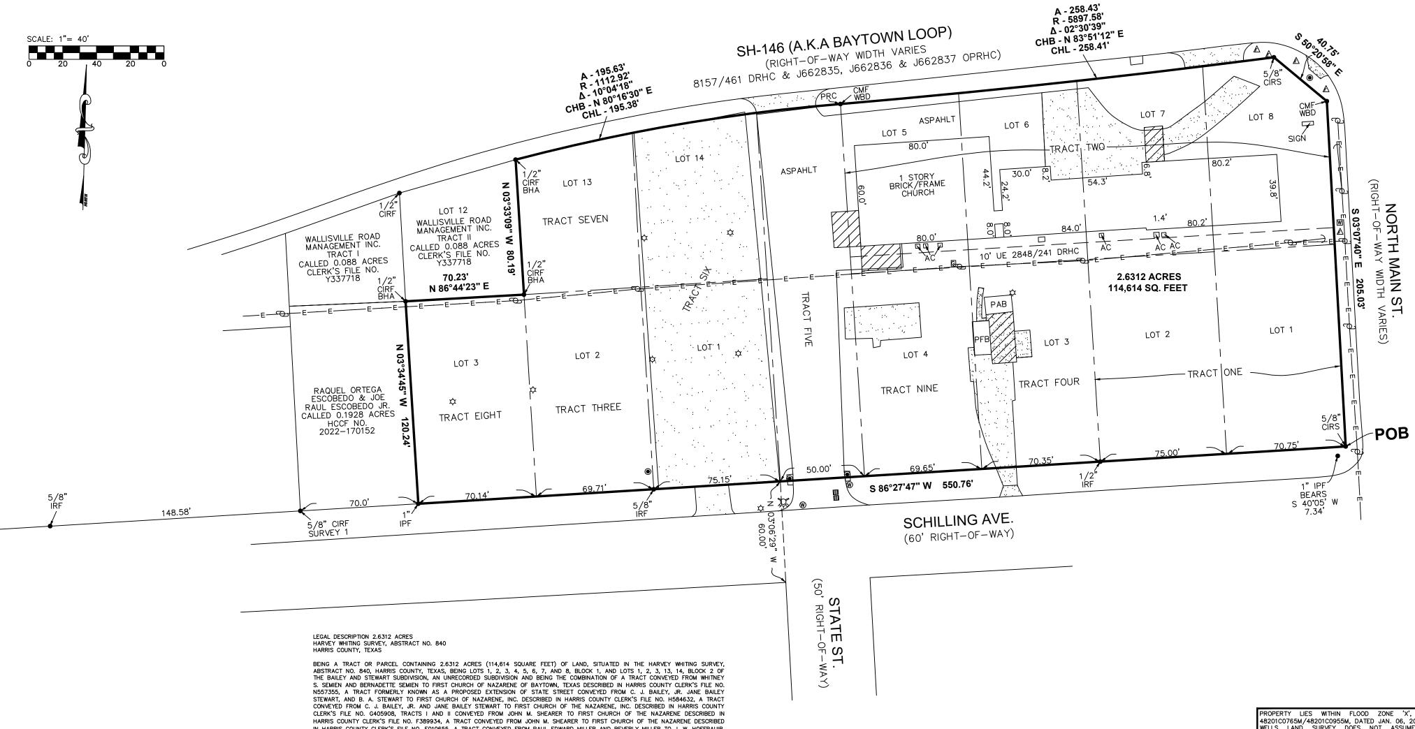
THE BEARINGS SHOWN HEREON ARE BASED ON THE TEXAS STATE PLANE COORDINATE SYSTEM, SOUTH CENTRAL ZONE, NAD 83.
