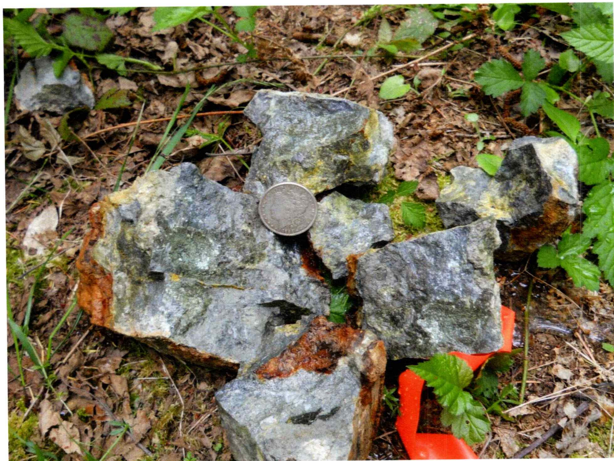
FIGURE 2: VMS (?) Mineralization on mine dump (80% sulfides) This sample contained 2.1 opt (64 g/t) gold. Silver dollar for scale.
