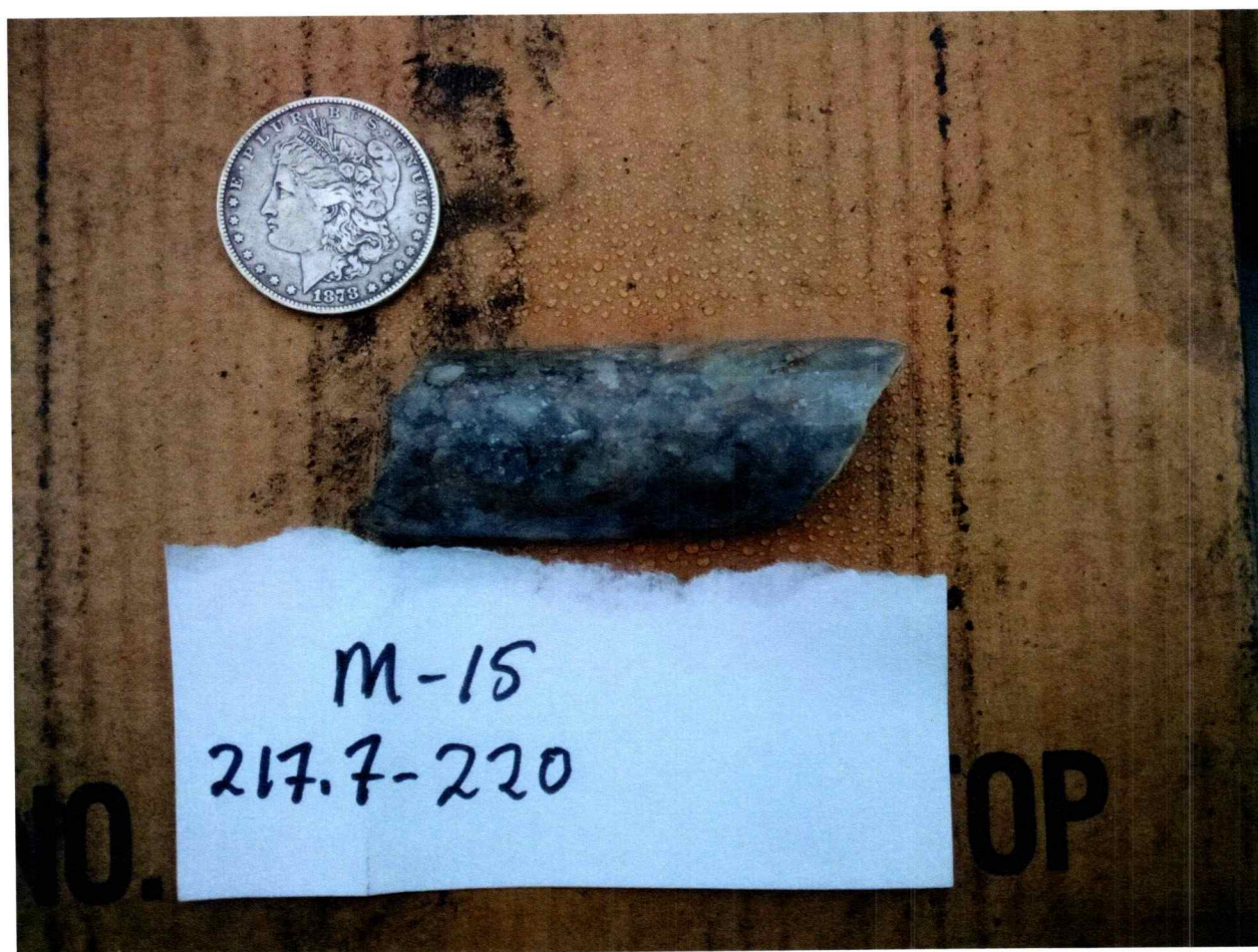
FIGURE 3: Typical mineralization seen in drill hole M-15 10% sulfides and 90% quartz. Silver dollar for scale.
