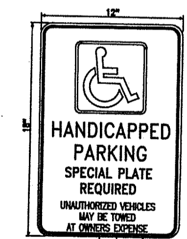
HANDICAPPED PARKING SIGN DETAIL (NO SCALE)
