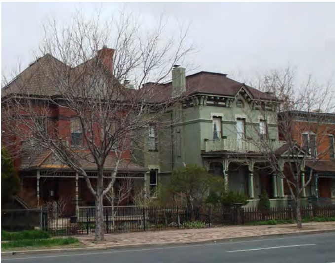
2. Typical streetscape within Curtis Park. Note the uniform front-yard setback of the Queen Anne structure on the left and the Italianate structures on the right, the at-grade front yards and the narrow side yards.
