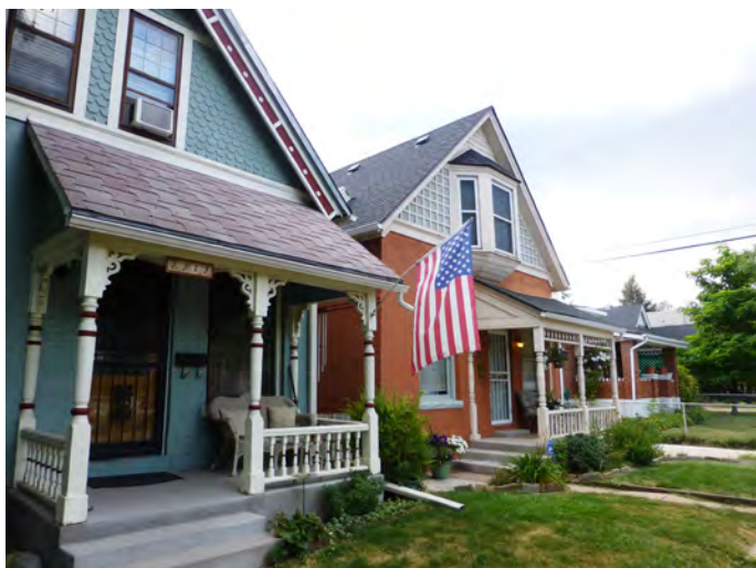
8. Typical one-and-a-half story Victorian brick cottages with front-facing roof gables and partial width front porches. These shed-roofed wooden porches feature wooden fretwork and spindle columns. Note the fishscale pattering and bay window in gable ends.
