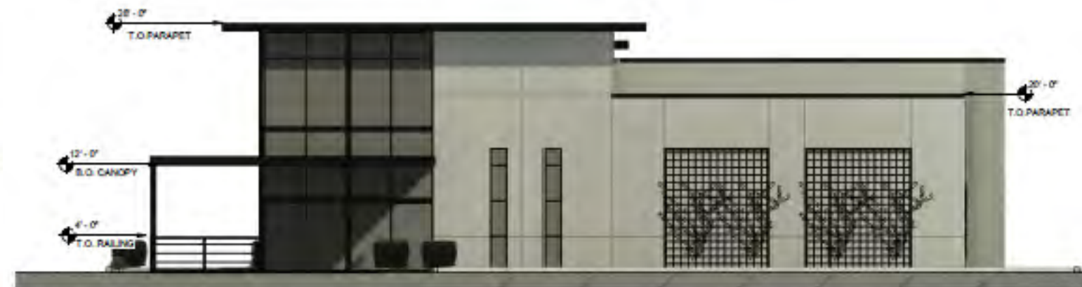
① PAD 6 EAST ELEVATION 1/8" = 1'-0"
