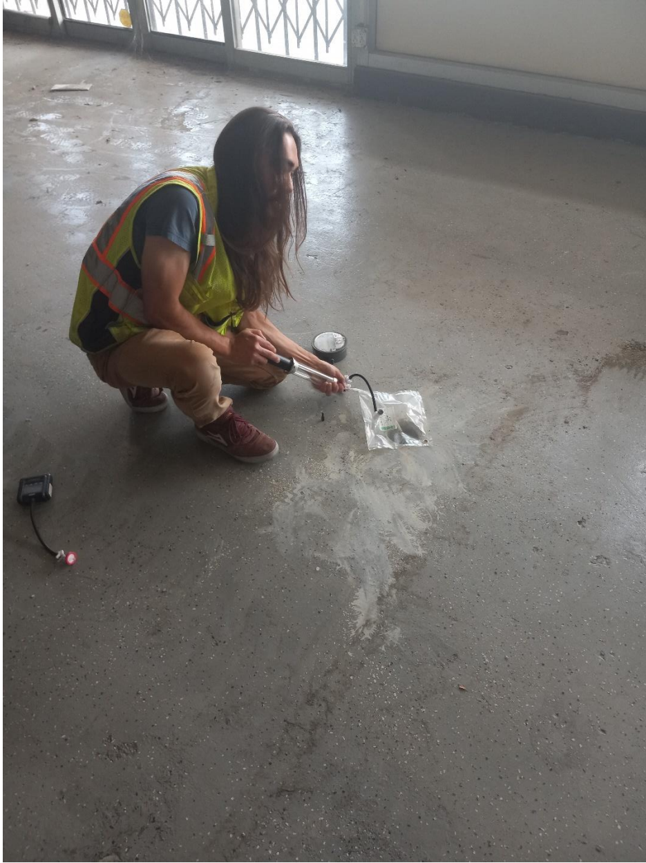
Photograph 3: View of the soil vapor sampling activities.
