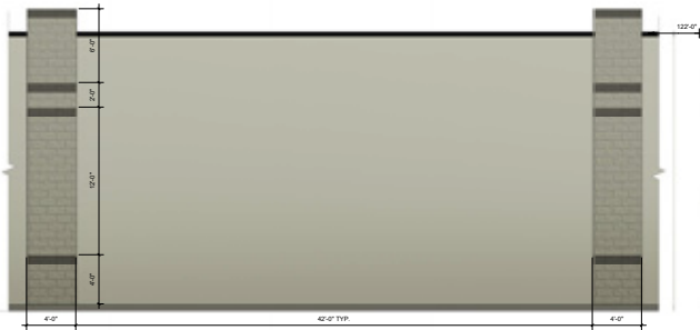
6 TYP MANCAVE PERIMETER BUILDING ELEVATION 1/4" = 1'-0"
