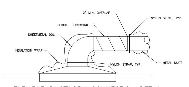
FLEXIBLE DUCTWORK CONNECTION DETAIL NO SCALE
