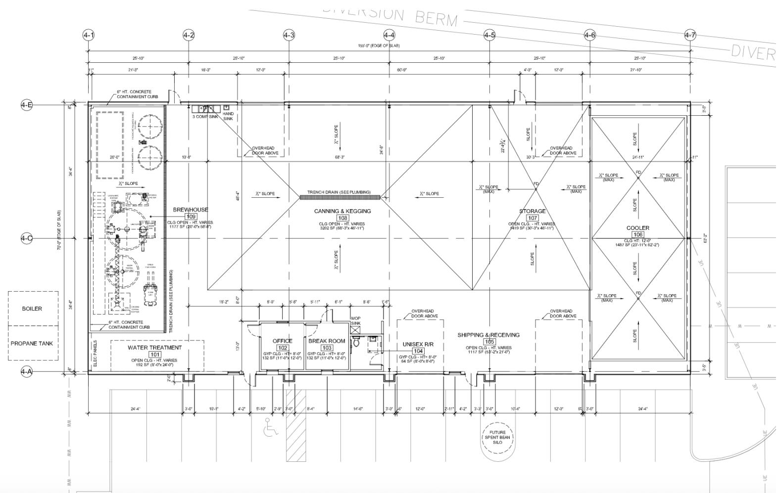
This space was engineered and built as a beverage/brewery facility. The slab slopes to floor drains in the production/brewery area and the canning/kegging area. Extensive electric for production equipment. Glycol header that is built for expansion. Climate-controlled office, break area and bathroom built out. 1,400 sf walk in cooler. Full list of brewery/production equipment available for purchase or owner finance.
