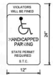
HANDICAP PARKING SIGN (B) CONNDOT #31-0629(P)
