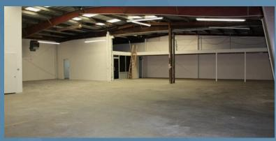
Property is situated on concrete slab floundation and features steel and masonry framed construction, painted cinderblock exterior and pitched corugated metal roof. The L-shaped configuration has 5500 Sq. Ft. of warehouse space behind the main office with 14' eaves and the 50' x 50' warehouse space in the rear has 16' eaves.
