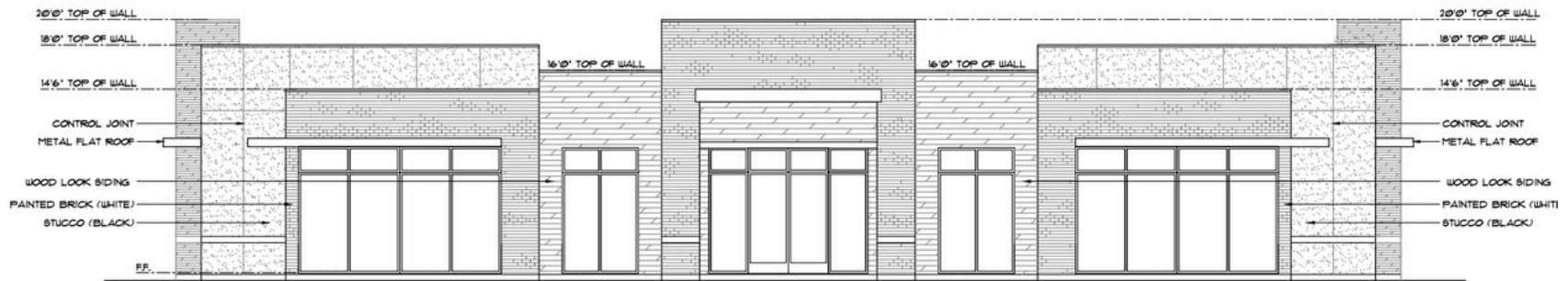
PRELIMINARY SOUTH ELEVATION 1/4" = 1'0"
