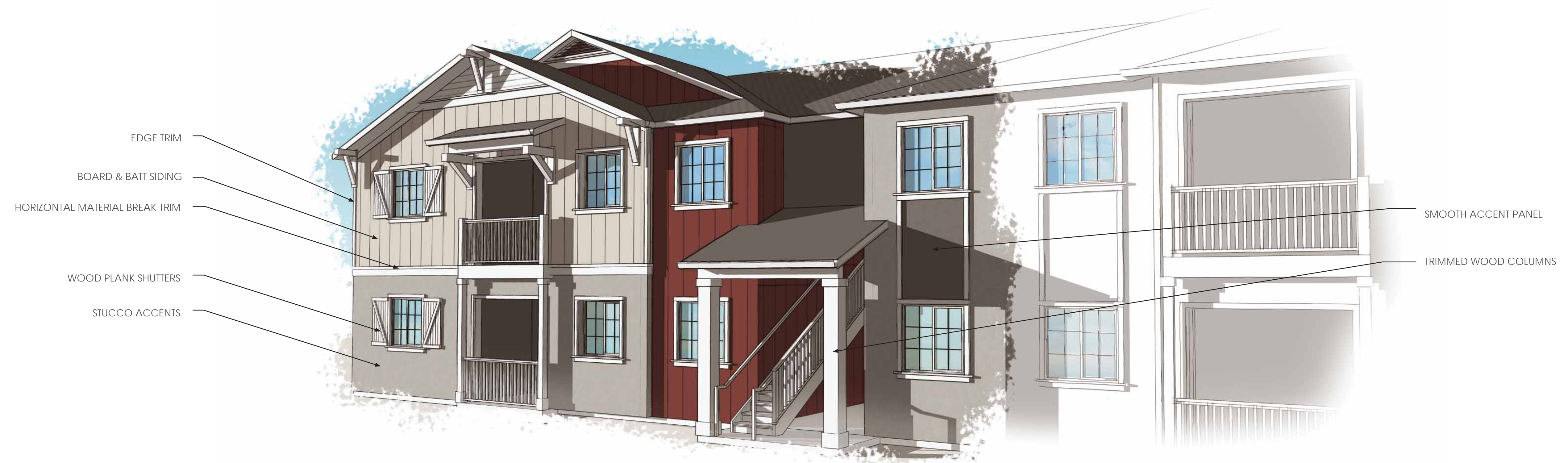
2 MULTI-FAMILY BUILDING INTERIOR STREET SIDE DETAILS
