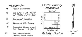
Note: All Bearings are referenced from True North observed at the Northeast Corner, Section 36, T17N, R1W.
