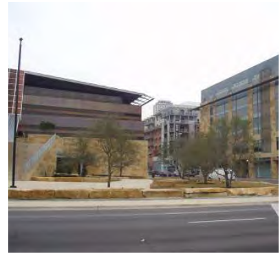
Figure 4-7: The Austin City Hall is set back from the street in some areas, while other non-civic buildings meet the street. This is a traditional urban design technique intended to emphasize the importance of civic uses.
