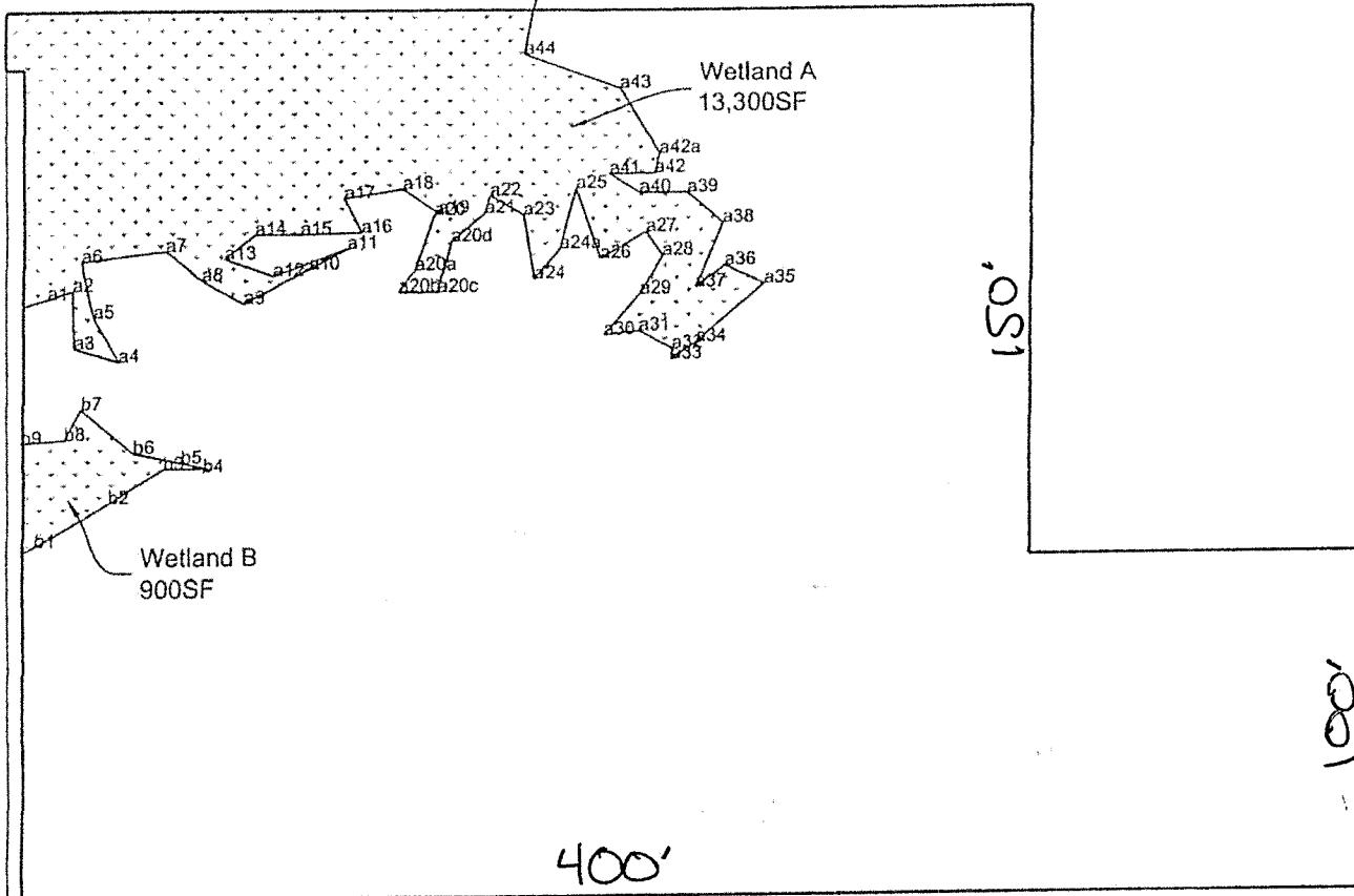
This map is intended to show wetland areas and their approximate relation to the subject site. These wetland and other features were mapped using sub-meter GPS technology and have a standard deviation of 1 meter $\pm$ . This does not constitute a boundary survey and should not be relied upon for determination of property lines. The approximate property lines indicated on the drawing are based on the description provided by the client.
