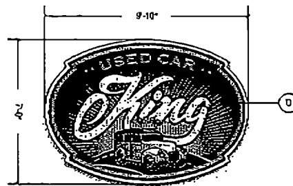
4 NORTH TOWER SIGN DETAIL (28 SQFT. TOTAL) SCALE: 1/4" = 1'-0"
