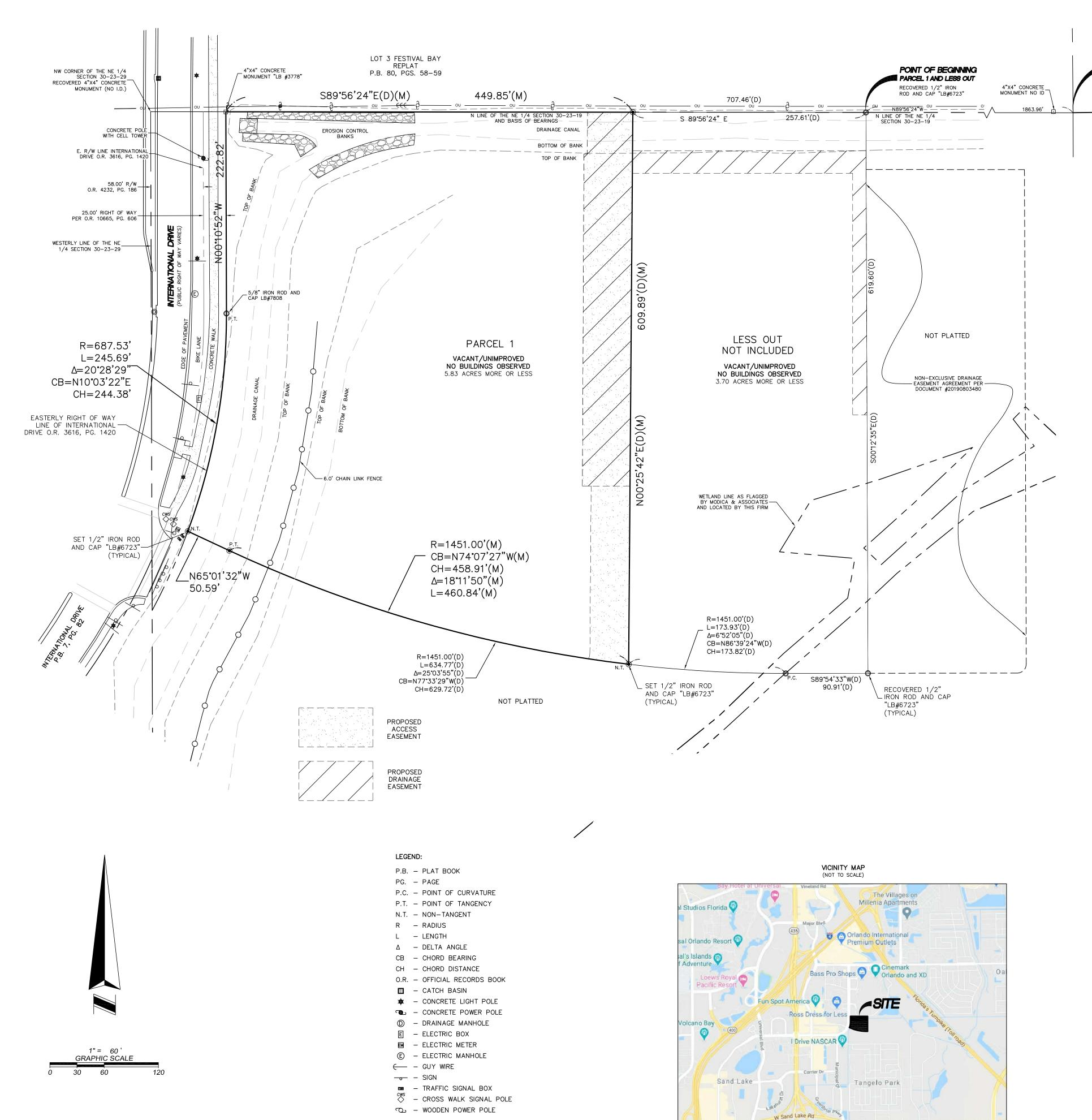
POINT OF COMMENCEMENT PARCEL 1 AND LESS OUT NE CORNER SECTION 30-23-29 CALCULATED PER RECOVERED WITNESS CORNERS (FALLS IN CANAL) 4"X4" CONCRETE MONUMENT FDOT NO I.D.
