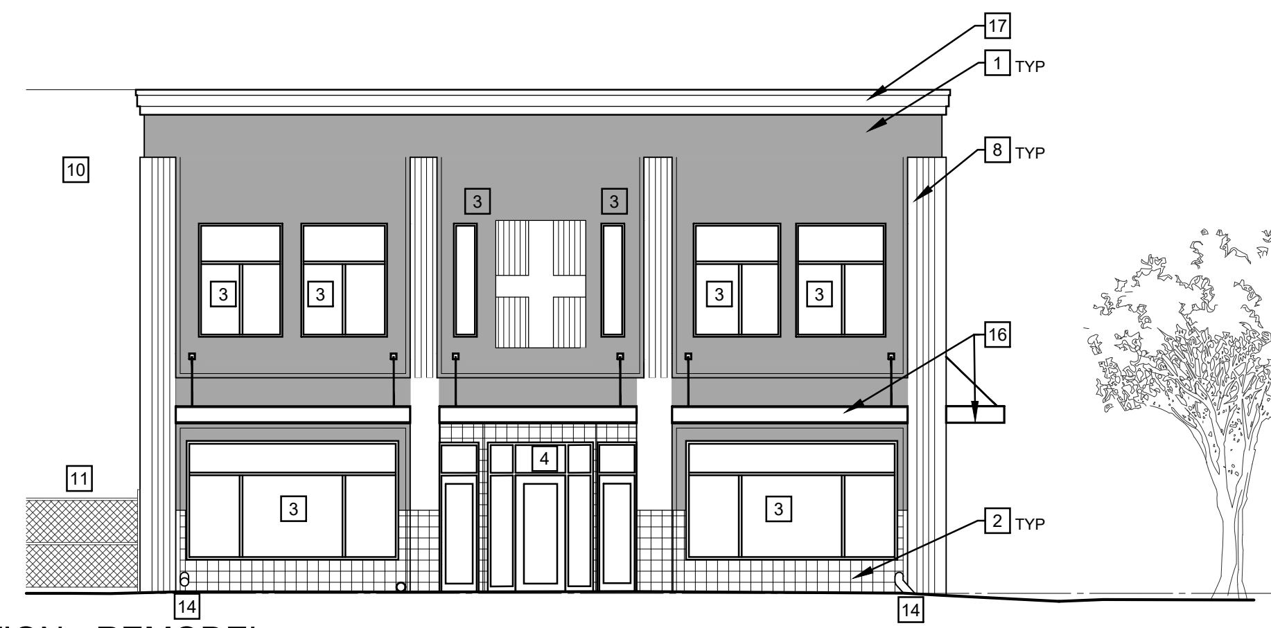
1 WEST ELEVATION - REMODEL SCALE: 1/8"=1'-0"
