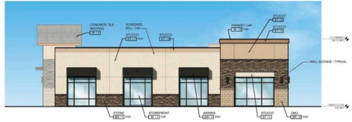
3 RIGHT SIDE (WEST) ELEVATION SCALE: 1/8" = 1'-0"
