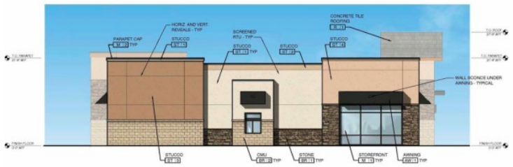
2 LEFT SIDE (EAST) ELEVATION SCALE: 1/8" = 1'-0"
