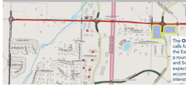
The Oak Street Extension and Overpass Project calls for the construction of a bridge that enhances the East to West connectivity in Rogers over I49 and a roundabout at the intersection of W. Oak Street and South Promenade Boulevard. The project is also expected to include a 10- to 12-foot-wide path to accommodate cyclists and pedestrians crossing the interstate.
