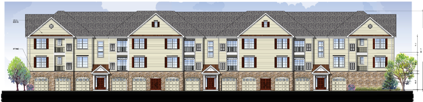
Front Elevation - Bldg Type B (29-Unit Bldg) Scale: 1/8"=1'-0"
