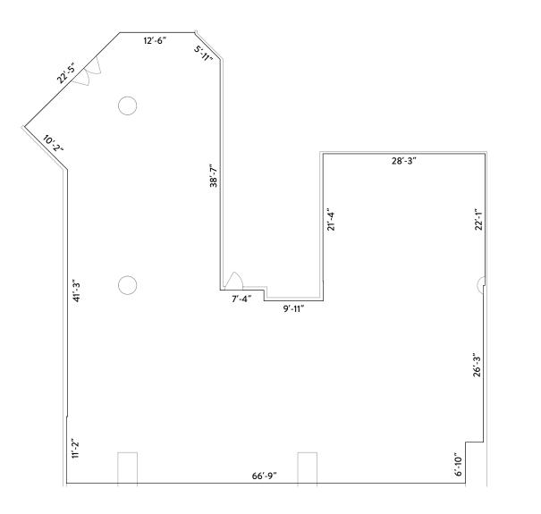
UNIT 235 **RETAIL AREA** 4,490 Square Feet **CEILING HEIGHT** Ranges from 8'1" to 13'5" POWER 225A, 120/208V, 42 Circuit Panel Fed from a 15 KVA transformer **HVAC** 4 Fan Coils Totalling 7 Tons **ECOLOGY UNIT** No WATER 1" Line (TBC) GAS Yes **SEWER** Yes
