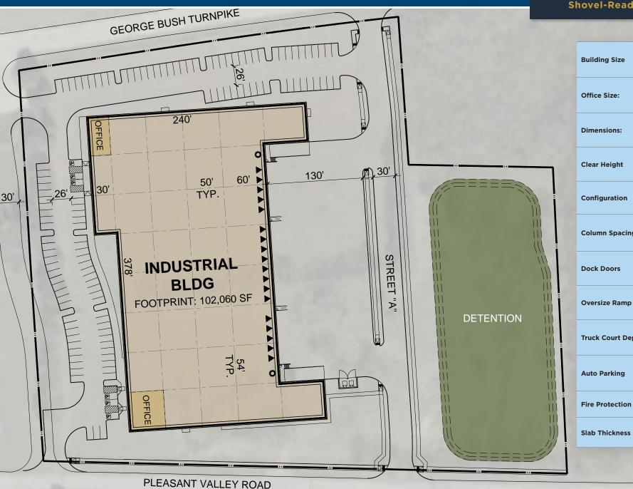
102,060 SF 2,181 SF 240' x 378' 32' Rear Load 54' x 50' **Column Spacing** (60' Speed Bay) 18 Oversize Ramp Doors **Truck Court Depth** 130' 127 **ESFR** 6"
