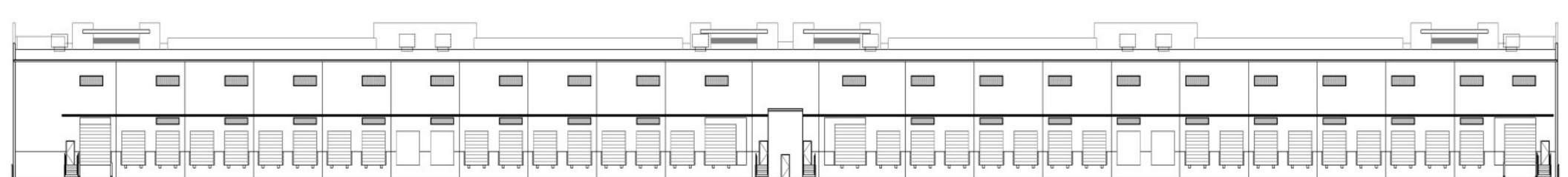
DRAGONFLY COMMERCE PARK TYPICAL TRUCK COURT/LOADING CONFIGURATION: BLDG. 2 REAR ELEVATION SHOWN
