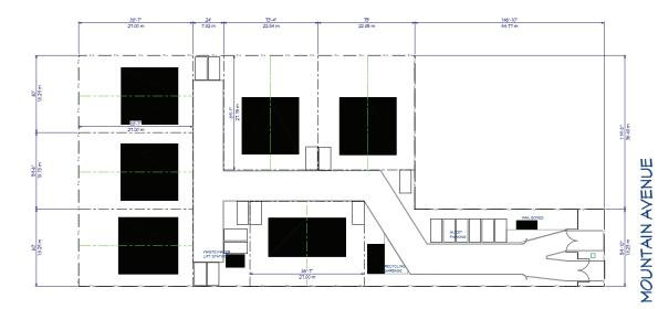
MF-1 MAX ALLOWED : SITE COVERAGE BUILDINGS - 40% SITE COVERAGE TOTAL WITH ALL IMPERMEABLE T0% FRONT SETBACK 4m SIDE SETBACK 51.0m REAR SETBACK 6m DISTANCE BETWEEN BUILDINGS 2m
