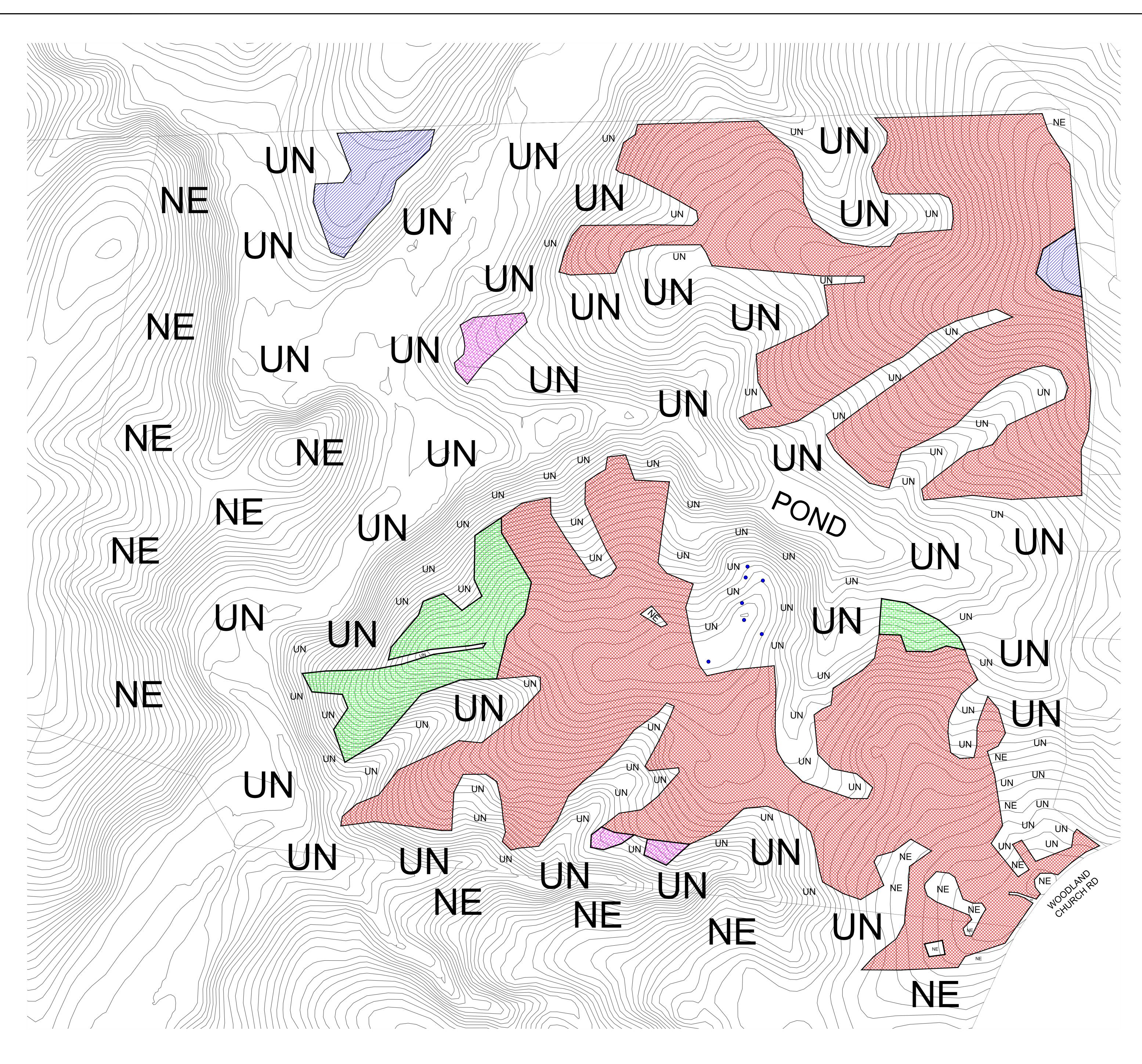
\*\*SUITABLE FOR PRELIMINARY PLANNING PURPOSES ONLY. SITE WILL REQUIRE APPROVAL BY THE COUNTY HEALTH DEPARTMENT AND/OR SOIL SCIENTIST ON A CASE BY CASE BASIS. THIS MAP SHOULD BE USED AS A GENERAL GUIDE. SOME ADJUSTMENTS WILL BE NECESSARY IN THE FIELD DUE TO SOIL VARIABILITY AND TOPOGRAPHIC IRREGULARITIES. THIS MAP ONLY REFLECTS EXISTING SOIL SUITABILITY FOR ON-SITE SEPTIC TANK SYSTEMS. SOME OTHER CONSIDERATIONS THAT AFFECT SITE SUITABILITY THAT SHOULD BE CONSIDERED IN DEVELOPMENT DESIGN ARE:
