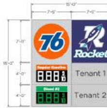
Custom High Rise Sign 22" PWM LED's | Split Electrical Per Tenant 85' Pole | Diameter TBD | Approximate Sizes
