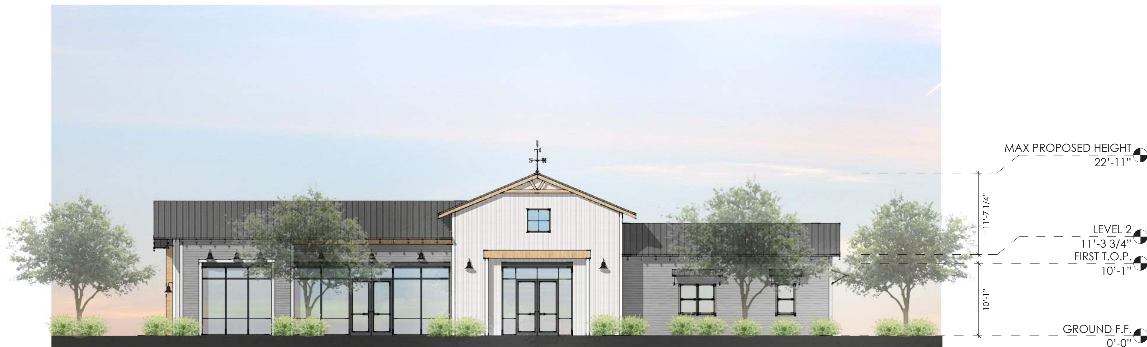
3 EAST ELEVATION-COMMUNITY BUILDING 1/8" = 1'-0" (24 X 36 SHEET)
