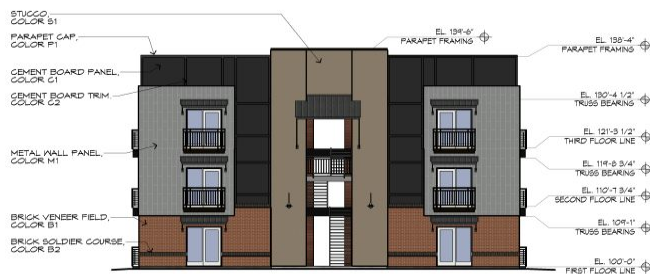
2 EXTERIOR ELEVATION BUILDING 1 & 2 SCALE 1/8" = 1'-0"
