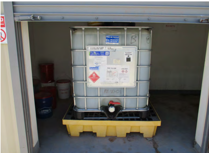
Photo 37 - View of the n-heptane rail tote on a spill pallet in the waste storage buildings.
