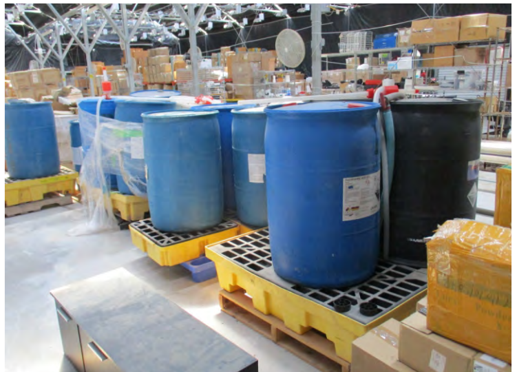
Photo 38 - View of drums of phosphoric acid on spill pallets in the Greenhouse 1 warehouse.
