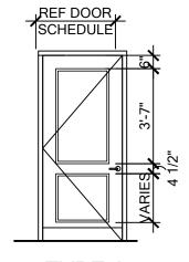
TYPE A -NEW FLAT PANEL DOOR ADD DECORATIVE MOLDING PER ELEVATION, PAINT -ALUMINUM FRAME **UNDERCUT DOOR 6"** FOR EXHAUST BLACK HARDWARE. PRIVACY LOCK SET
