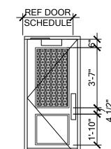
TYPE B -NEW DOOR WITH **DECORATIVE GLASS INSERT METAL GRID** GLASS WITH FROSTED GLASS. REVIEW INSPO **IMAGE PROVIDED BY** ARCHITECT. PAINT -ALUMINUM FRAME -BLACK KICK PLATE BLACK MOP PLATE -BLACK CLOSER
