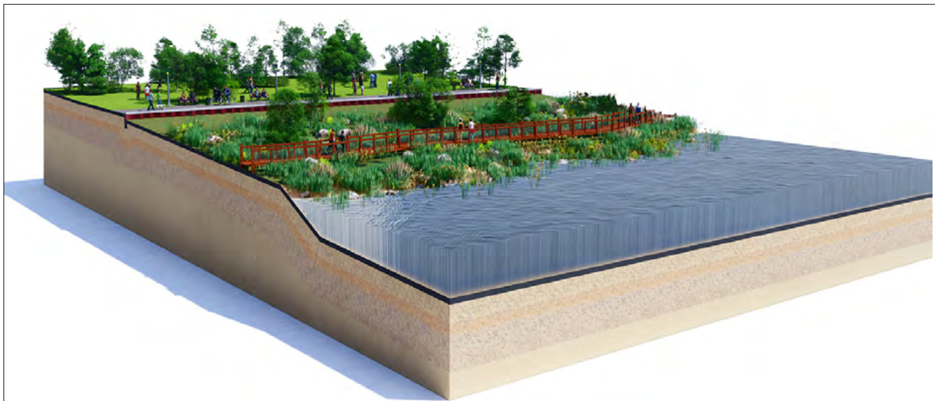
Living Shoreline Section (above) and perspective View (below). Although the height of the wall has not been set, these drawings illustrate the concept for the retaining wall and the waterfront walkways on pilings. There will be a railing on the retaining wall as it is likely to be at least 5' high. Click on images for larger views.
