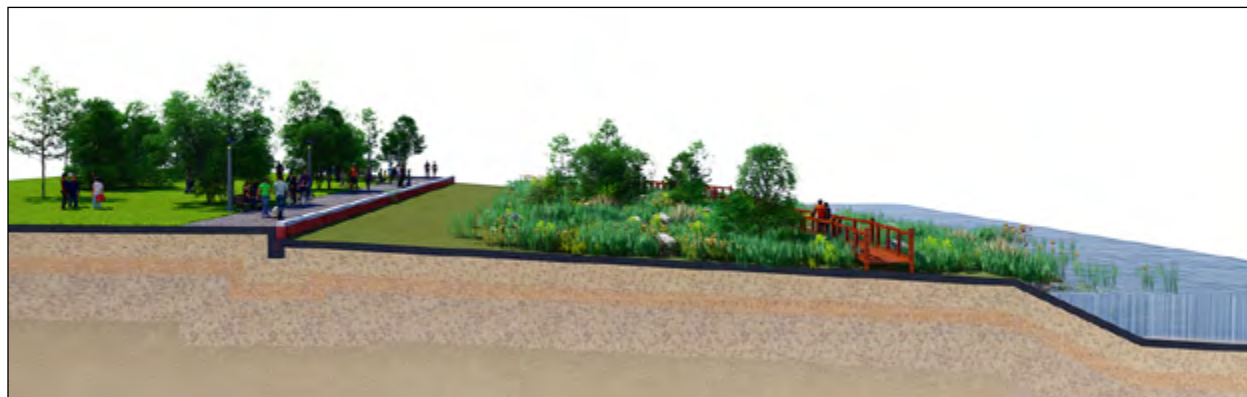
Living Shoreline Section (above) and perspective View (below). Although the height of the wall has not been set, these drawings illustrate the concept for the retaining wall and the waterfront walkways on pilings. There will be a railing on the retaining wall as it is likely to be at least 5' high. Click on images for larger views.
