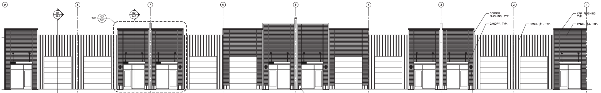
03 ENLARGED ELEVATION: Horizontal Wall Panels 1/4" = 1'-0"
