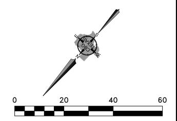
BEARINGS SHOWN ARE BASED ON NAD 83 TEXAS SOUTH CENTRAL ZONE. EASEMENTS AND BUILDING LINES ARE BY RECORDED PLAT UNLESS OTHERWISE
