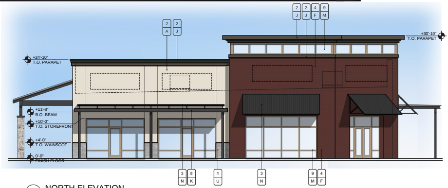
4 NORTH ELEVATION SCALE: 1/8"=1'-0"
