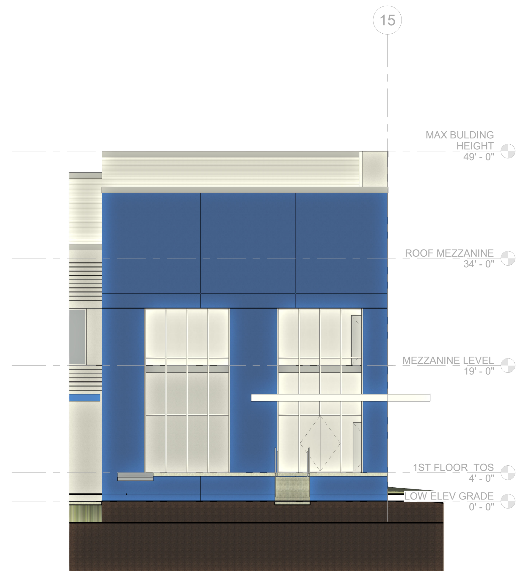
3 WEST ELEVATION - ENLARGED CORNER 1/8" = 1'-0"
